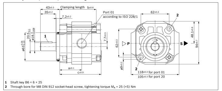
Туре **Material numbers** b Port standard Port optional PGF2-2X/ **006** R **A** 01VP2 R900932272 46 76 87.2 01 20 **008** R **A** 01VP2 R900564037 47.8 79.5 90.7 01 20 **011** R **A** 01VP2 R900568523 50.5 85 96.2 01 20 **013** R **A** 20VP2 R900032712 53 90 101.2 20 01 20 **016** R **A** 20VP2 R900932275 55.5 95 106.2 01
